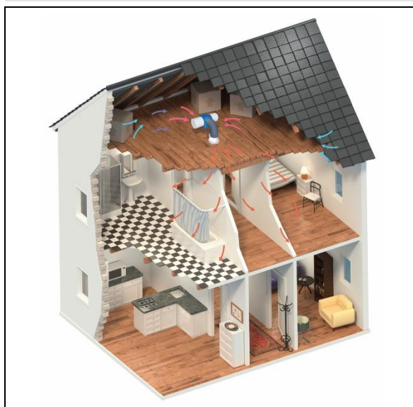
Figure 1 Loft-mounted ventilation unit
